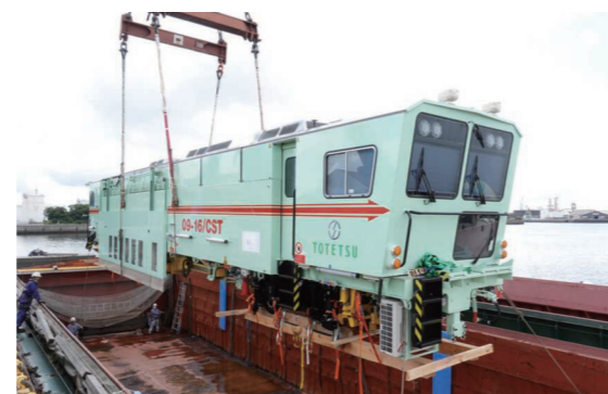
Multiple tie tamper, loading scene
